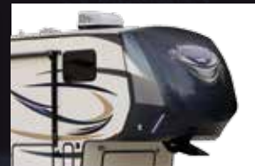
Painted gel coat fiberglass front cap with light strips on Lite Series Travel Trailers and Fifth Wheels, won't fade, chalk or crack
